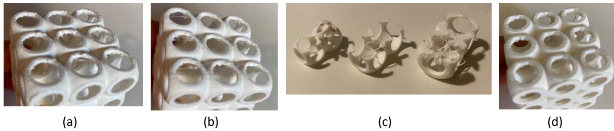
Figure 2: Examples of defects during 3D printing: (a) curly filaments in the top of the holes due to overhang; (b) strings inside the part; (c) different scale factors; (d) a sample with few defects
