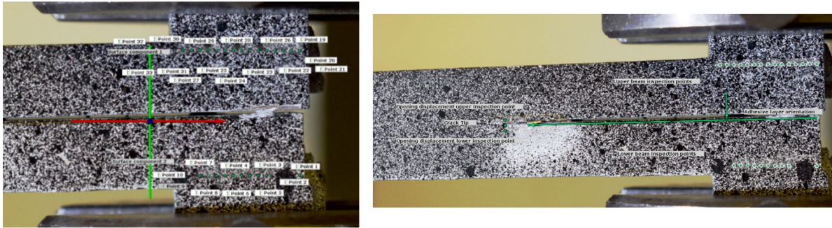
Figure 3: Marked points in the DIC software to calculate the loading point rotations (left) and to determine the CTOD (right).
