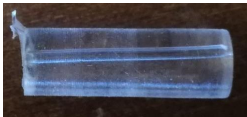
Figure 2: Flexible transparent PDMS device showing the interior microchannel
