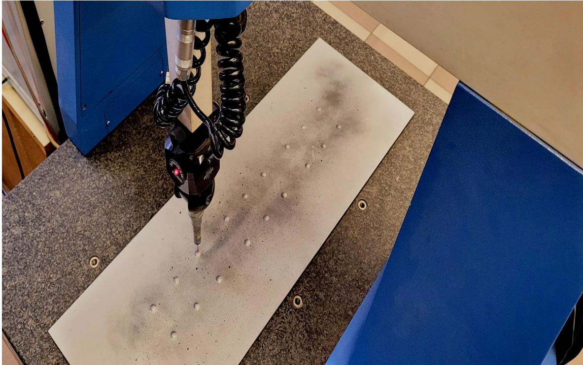
Figure 10: The process of measuring deformation heights using the coordinate measurement machine
