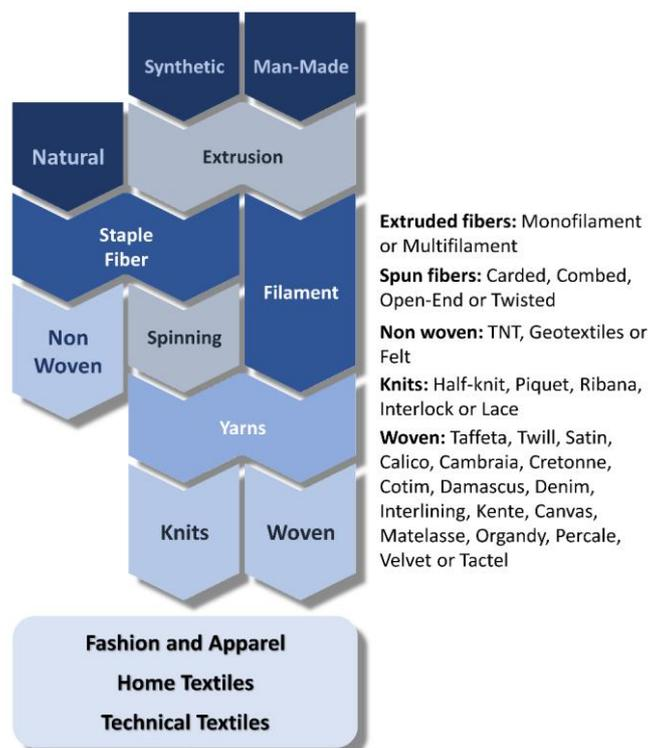
**Figure 1:** Representative scheme of several types of yarns and textile structures
