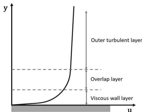
Figure 2: Typical velocity distributions in turbulent flow near-wall
