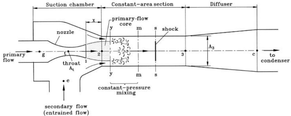
Figure 1: Ejector flow demonstration scheme (Huang et al. 1999)
