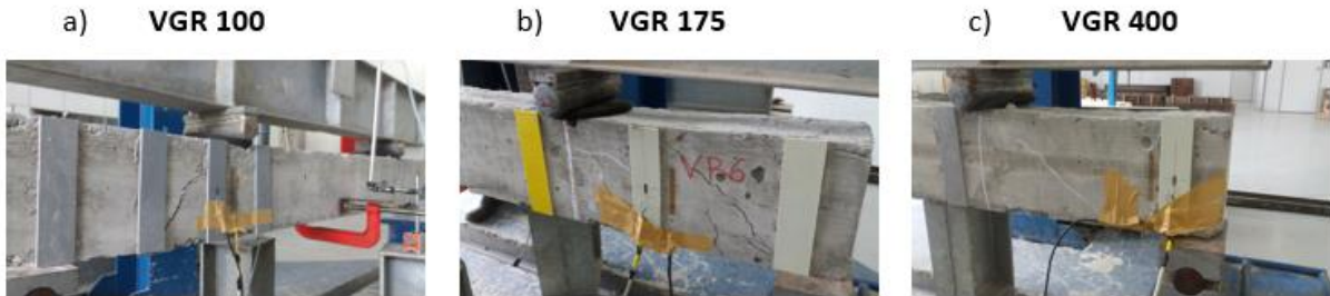
Figure 11: Positioning of the strain gages on the beams: a) VGR 100; b) VGR 175 and c) VGR 400
