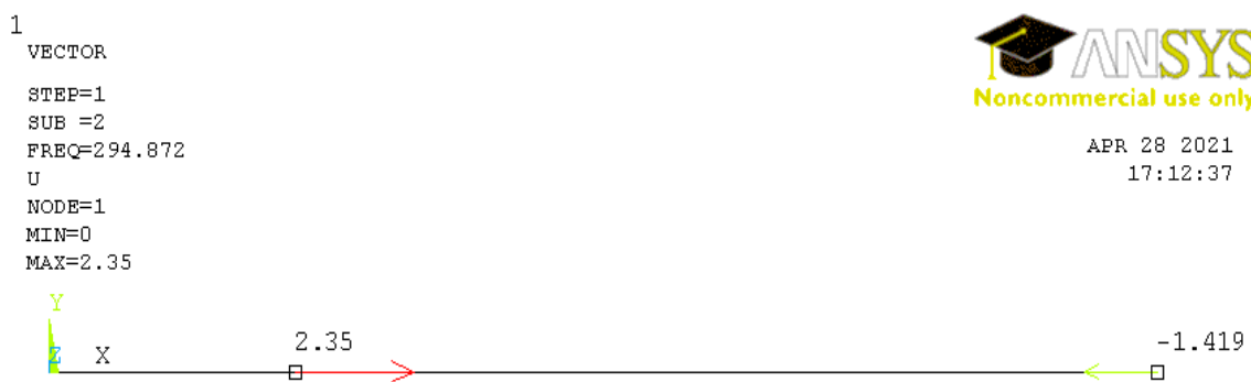
Figure 5: Second mode shape plot; V-shaped crack; crack depth 5 mm; location 80 mm
