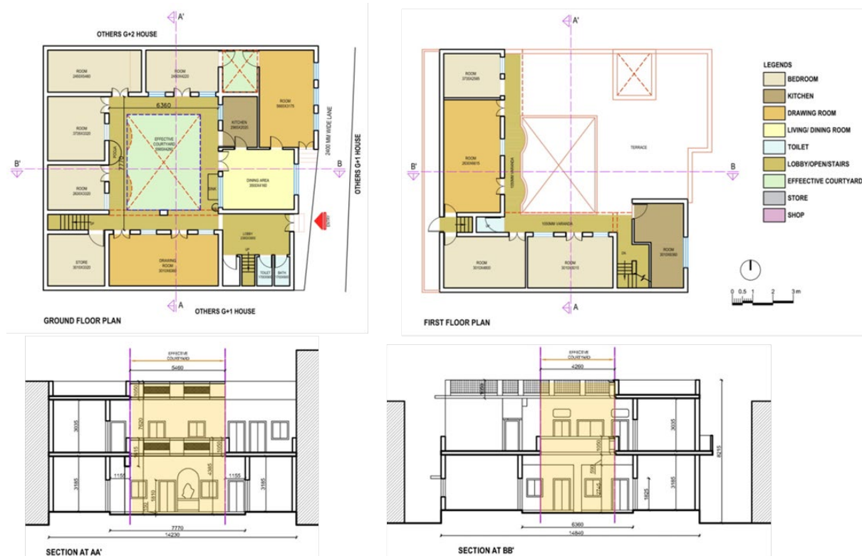
Figure 3: The figure above depicts the ground and first-floor plan space arrangement and effective proportions of the courtyard of House 1
