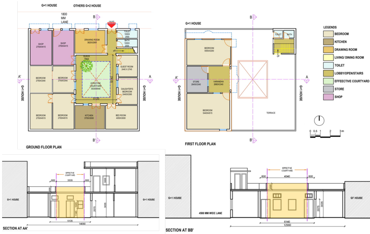
Figure 4: The figure above depicts the ground and first-floor plan space arrangement and effective proportions of the courtyard of House 2
