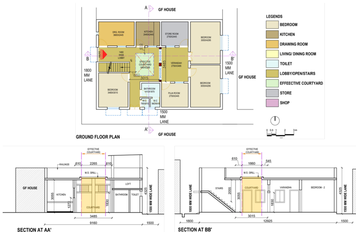
Figure 7: The figure above depicts the ground and first-floor plan space arrangement and effective proportions of the courtyard of House 5
