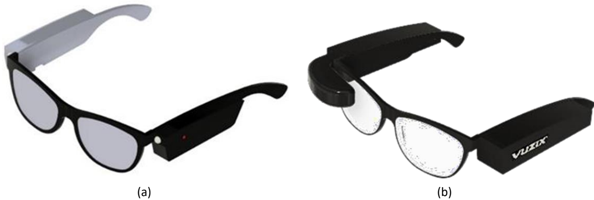
Figure 5: Smart Glasses CAD model: a) Imported model. b) Redesigned model (Vuzix M300).
